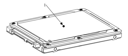
Figure 3.4 Surface cover temperature measurement points
